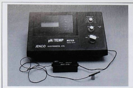
Fig 1 The pH meter, offset, and electrode used to measure the pH of the bleaching solution, plaque, and saliva.
