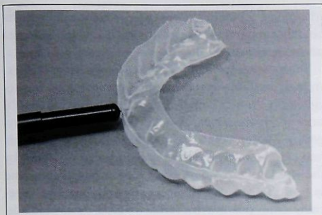
Fig 3 Insertion of the electrode through a small hole in the bleaching guard to measure changes in the pH of the bleaching solution during bleaching.
